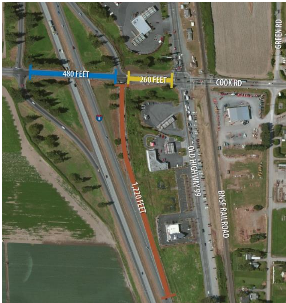
Figure 3-3. Roadway Storage Lengths for Queuing Vehicles
