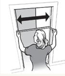
**Door Clear Width** Open the door 90 degrees, measure from the face of the door to the edge of the door stop.
