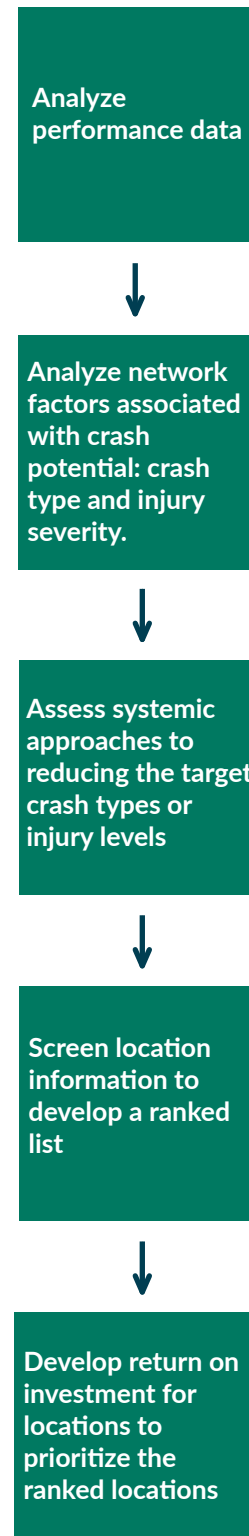
Exhibit 13. I-2 Safety Program General Process Flow
